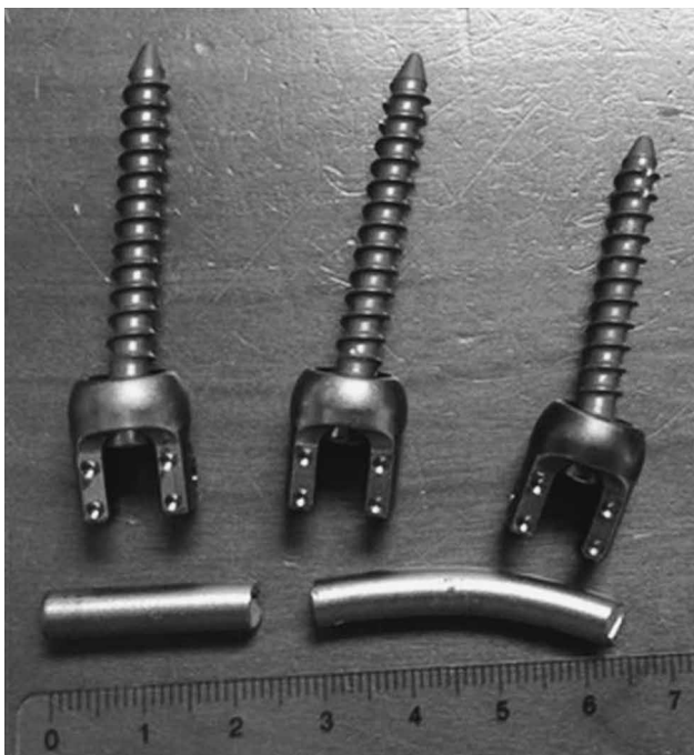
Figure 5 Broken rod after removal.
